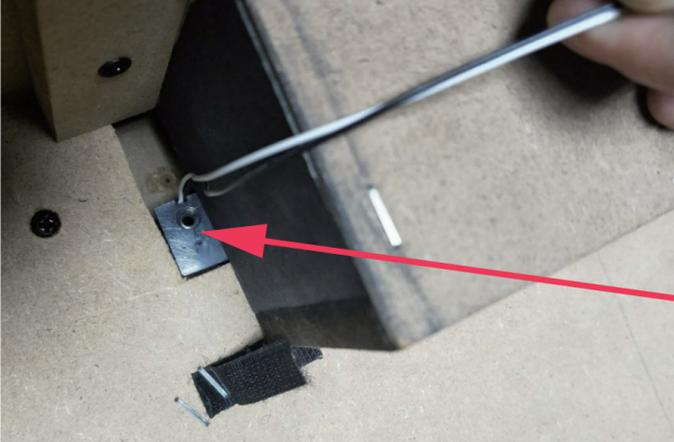
3. Unscrew the screw of the IR sensor.
