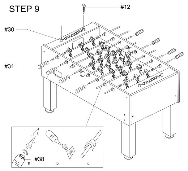
• Spray the lubricant(#38) into a clean, soft cloth and then use the cloth to wipe the player rods where they come into contact with the bearings. See above.
